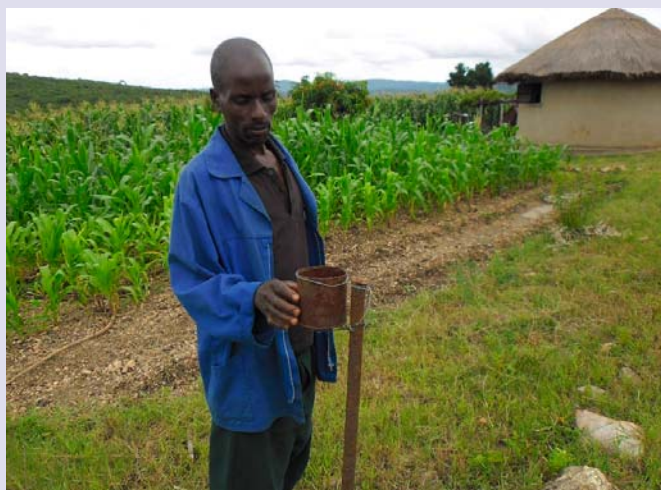
4. A farmer practicing conservation agriculture (CA) in Shurugwi with an improvised rain gauge made from an empty tin.
